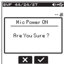
Select the **F3**  button for plug-in-power microphones, or **F2**  button for other microphone types.
