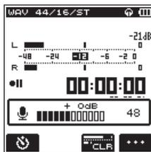
To obtain higher quality, it is recommended to set at the maximum recording level. As a guideline, adjust the input level until the **-12dB** indicator lights in green to obtain the optimum level. To prevent possible distortion from excessively large input volume, reduce the input level when the **PEAK** indicator lights in red.
