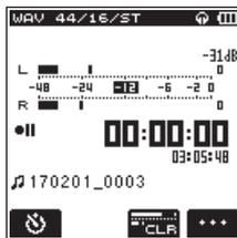
2. Use the **INPUT LEVEL** volume to adjust the input level. The input level setting meter will pop-up at the bottom of the display.
